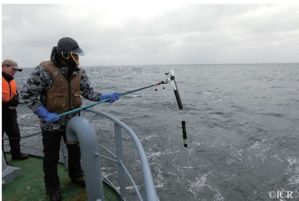
Photo 11. Oceanographic observation using XCTD.
